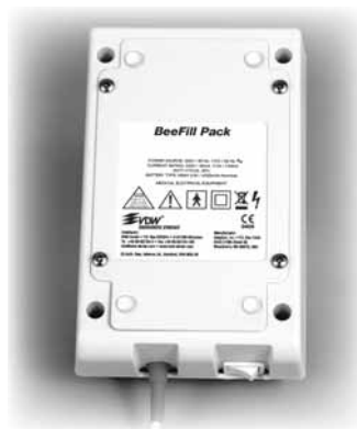
Figure 4 – Battery Pack Cover Plate Installed
